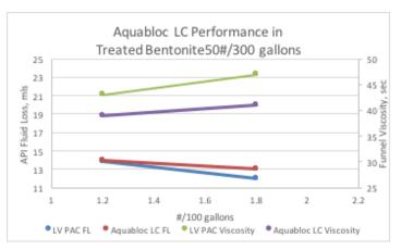
Performance can be reduced when used in systems with greater than 100,000 PPM chlorides and or 1,000 ppm calcium. Use of untreated bentonite is recommended to improve fluid loss and viscosity performance.
