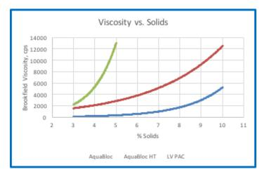
AquaBloc and AquaBloc HT both deliver excellent fluid loss without the viscosity penalty of PACs. This allows the driller to use more of the additive if additional fluid loss is desired without exceeding the functional viscosity of the fluid.
